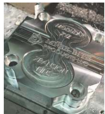
Op 2 including c'bore on same fixture
